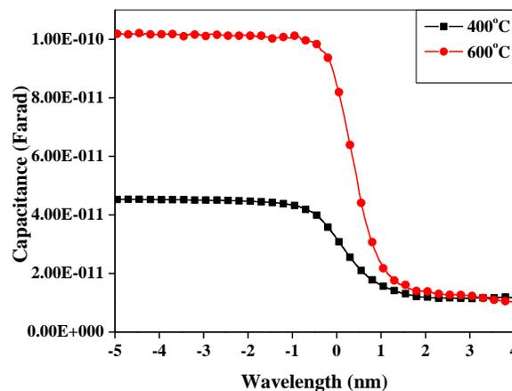
Fig.6.C-V characteristics of CeO<sub>2</sub> thin films annealed at (a) 400°C (b) 600°C for 3hr in air ambient.
