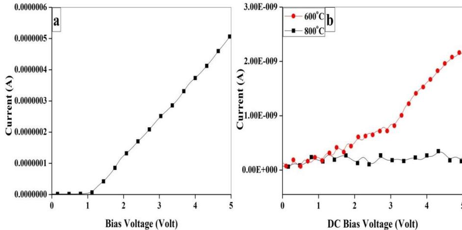
**Fig. 8 (a,b):** I-V characteristics of CeO<sub>2</sub> thin films conventionally annealed at (a) 400°C (b) 600°C and 800°C for 3 hr
