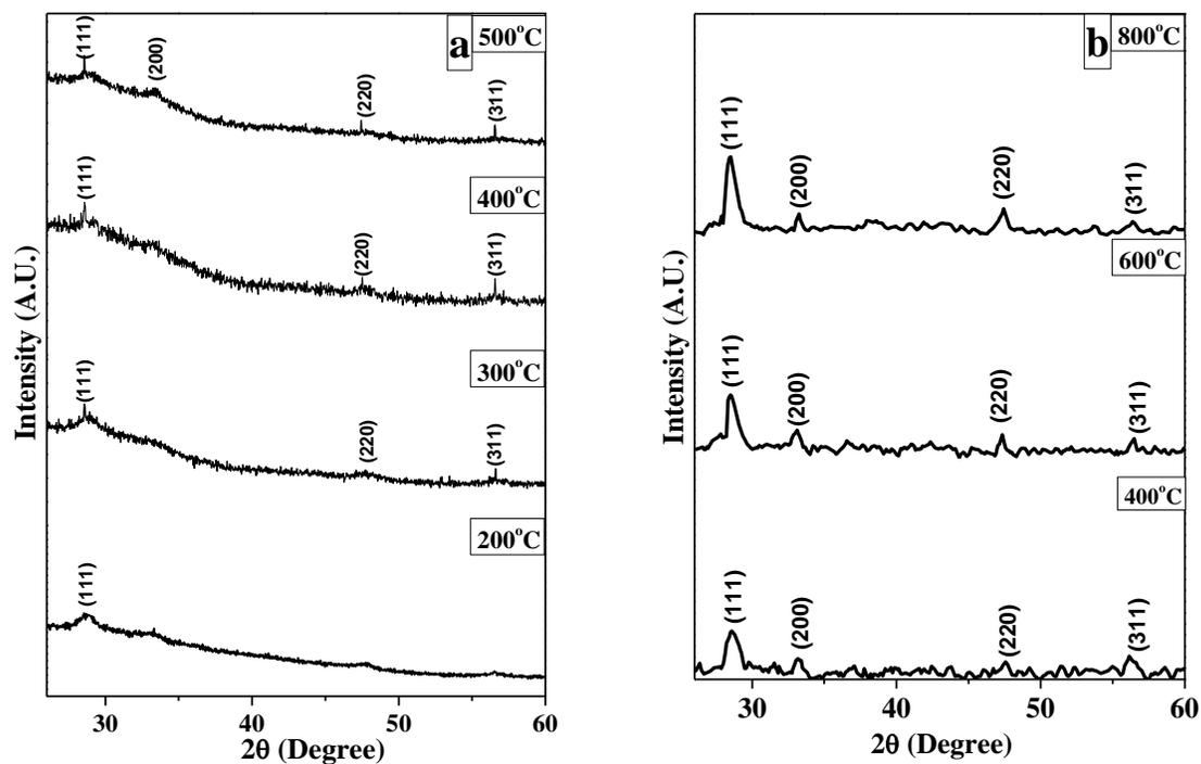
**Fig.1(a, b):** XRD pattern of CeO<sub>2</sub> thin films coated on (a) glass substrates and annealed at different temperatures for 1hr (b) silicon substrates and annealed at different temperatures for 3hr.
