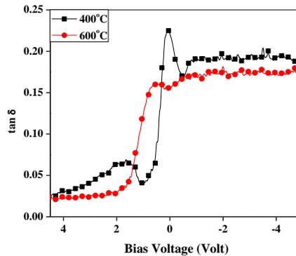
Fig.9. tanδ-V plot of CeO<sub>2</sub> films annealed at 400°C and 600°C for 3hr in air ambient.
