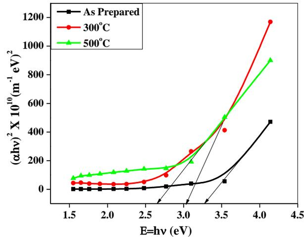
Fig.5. Optical band gap estimation of the as-prepared and annealed CeO<sub>2</sub> thin films.
