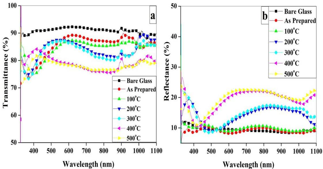
**Fig.4** (a) Transmittance spectra (b) Reflectance spectra of CeO<sub>2</sub> thin films deposited on glass and conventionally annealed at various temperatures
