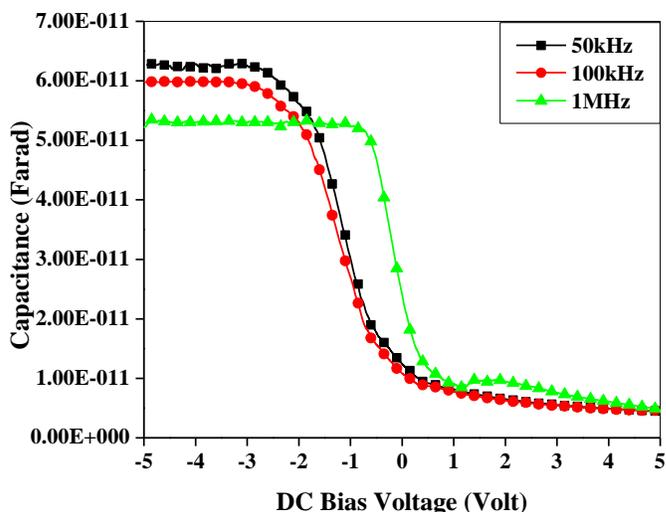
Fig.7. Frequency dependence of accumulation capacitance of CeO<sub>2</sub> thin films annealed at 800°C for 3hr in air ambient.
