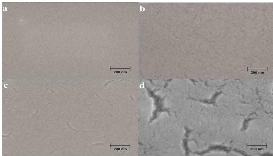
**Fig. 2 (a-d):** SEM images of  $\text{CeO}_2$  thin films annealed at (a) 400°C/1hr (b) 500°C/1hr (c) 600°C/3hr (d) 800°C/3hr
