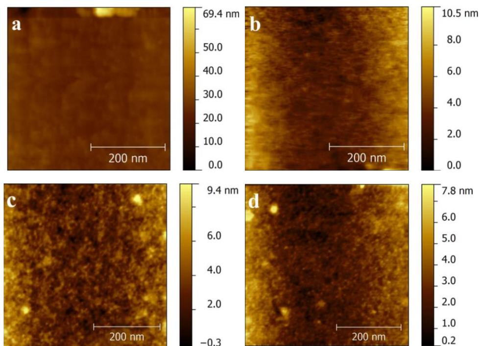
**Fig.3 (a-d):** AFM micrographs of CeO<sub>2</sub> thin films conventionally annealed at (a) 400°C/1 hr (b) 500°C/1 hr (c) 600°C/3hr (d) 800°C/3hr
