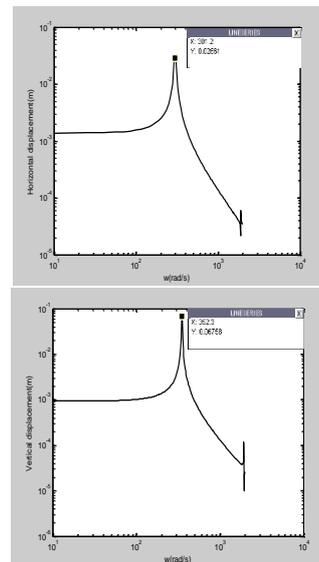
Fig.4. Horizontal and vertical steady-state responses of cracked rotor at 0.225m from left end (a=1)
