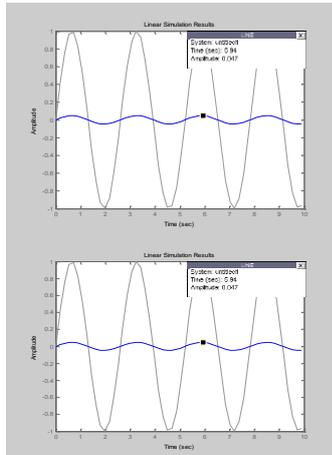
Fig.5. Horizontal and vertical time response signal of cracked rotor at 0.225m from left end (a=1)
