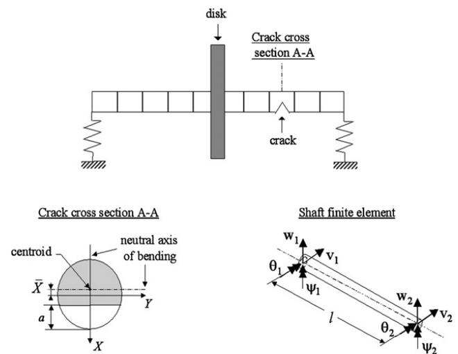
Fig.1. Rotor system and crack model cross-section.
