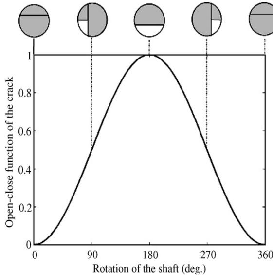
Fig.3.: Opening and closing of the crack
