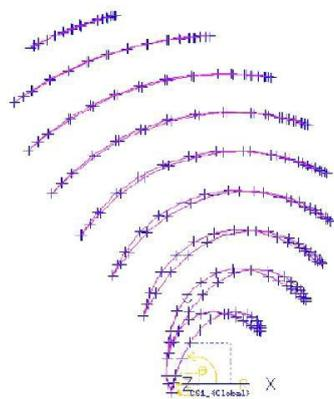
Fig 4: Construction of hydrofoils by joining of points on surface of the blade.
