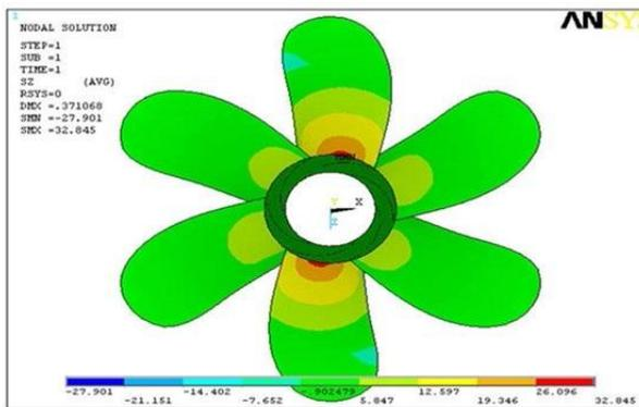
Fig 7.Max. Normal stress of Al propeller
