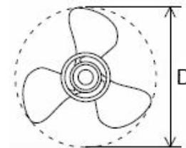
Fig 2. Diameter of the Propeller
