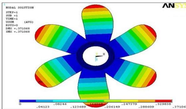
Fig 6.Max deflection of Al propeller
