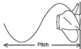
Fig 1. Pitch of the Propeller
