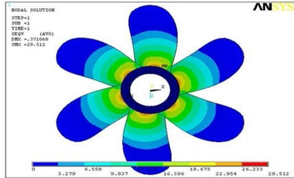
Fig 8.Max. Von mises stress of Al propeller
