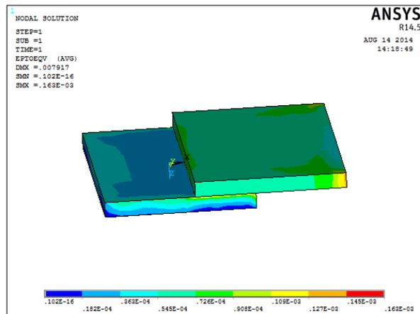
Fig6: strain for lap joint
