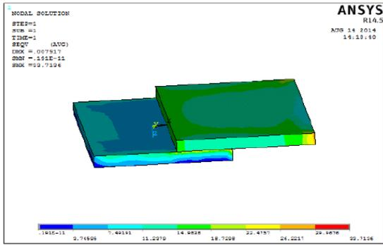
Fig 5: Stress for Lap joint
