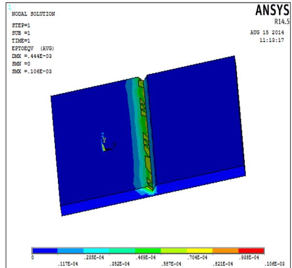
Fig3:strain for Tee joint
