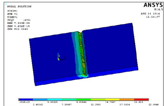
Fig 4: Stress for TEE joint
