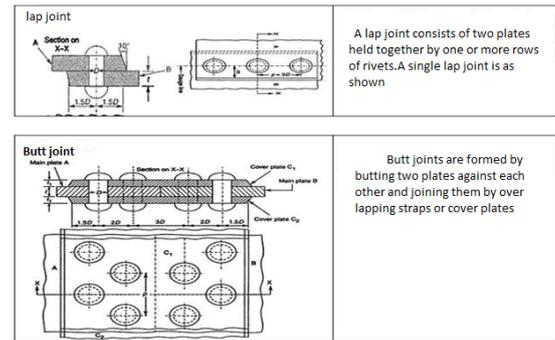
Fig:3 Types of joints.
