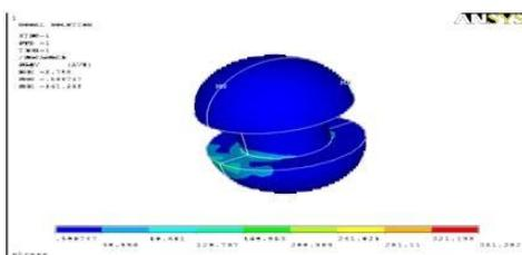
Fig:4 The stress distribution of a rivet without adhesive
