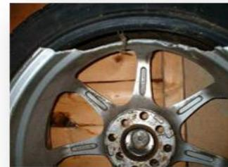
Fig.2 FATIGUE FAILURE ON A WHEEL RIM
