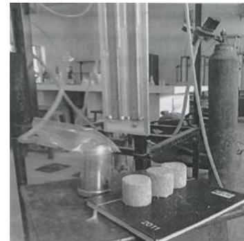
Fig 3: Specimen preparation using CO<sub>2</sub> Process
