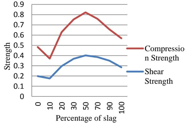
Fig 9: Shear and compression strength test graph
