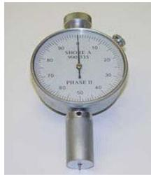
Fig 5: Hardness Tester
