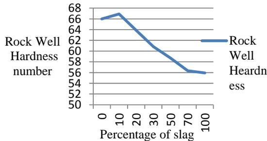
Fig 12: Rockwell Hardness graph
