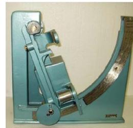
Fig 8: Universal Sand Strength testing machine
