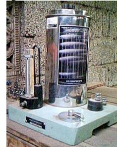
Fig 6: Standard permeability meter
