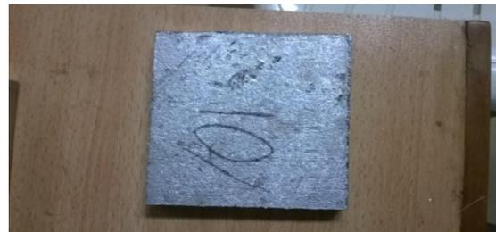
Fig 8(b): Al - 10% of SiC hardness test specimen
