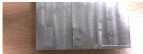
Fig 8(c): Al - 15% of SiC hardness test specimen
