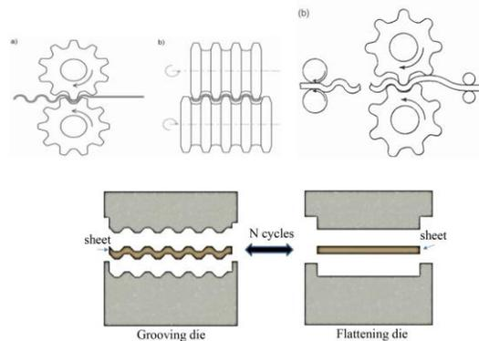
Fig.3. Different types of RCS process
