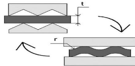
Fig.2. Repetitive Corrugation and Straightening Process
