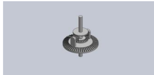
Fig 6: ASSEMBLY OF DIFFERENTIAL GEAR BOX
