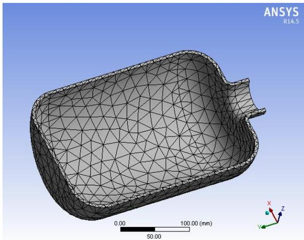
Figure 2: Mesh model of the component
