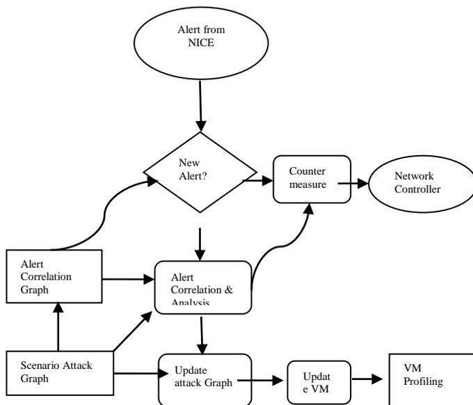
Fig . Workflow for Attack analyzer.
