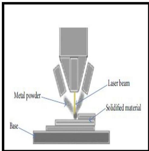
FIGURE 5: Laser engineered net shaping
