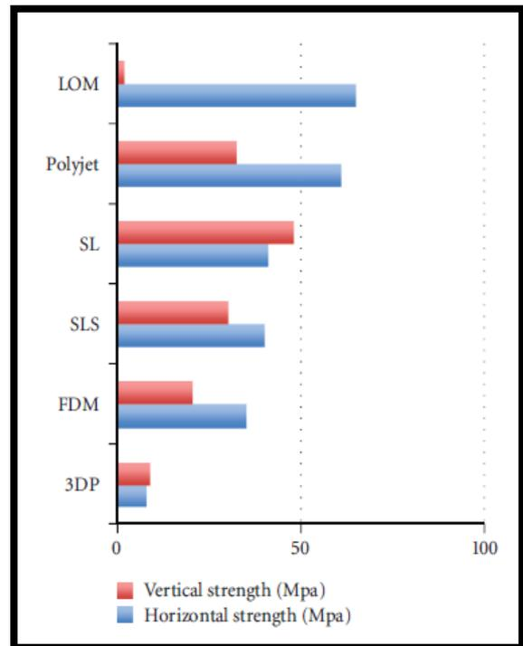
FIGURE 7: Tensile strength of 3-D printing process
