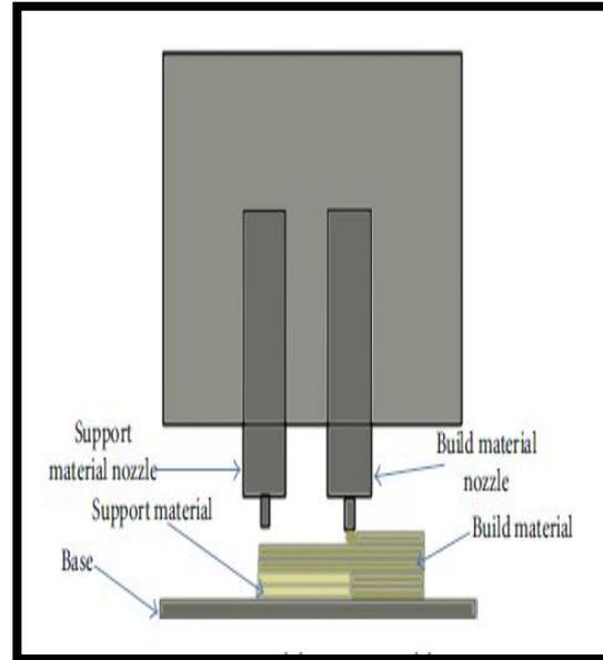
FIGURE 4: Fused deposition modeling
