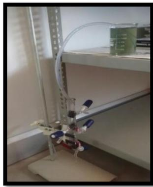
Fig-5 fixed bed column with wastewater
