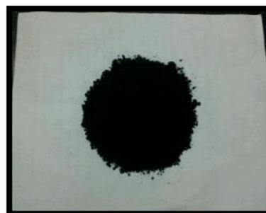
Fig -2 activated waste tire rubber
