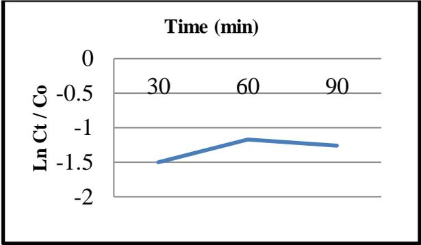
Fig – 7 Adam-Bohart model for Cu (II) adsorption
