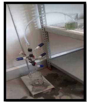
Fig -6 fixed bed column with wastewater
