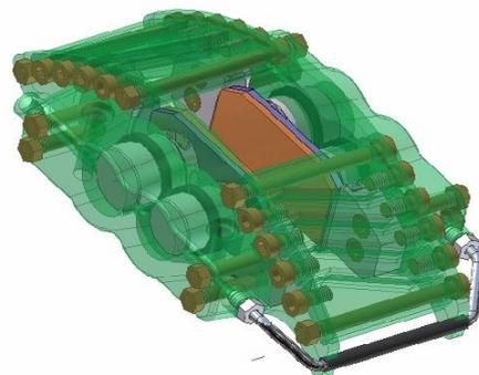
Fig: 5 Internal structure of modular brake caliper assembly
