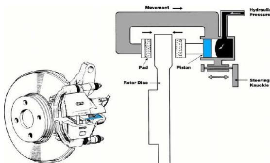
Fig: 2 Disc brake assembly
