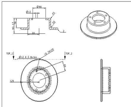
Fig: 9 Draft model of a solid disc
