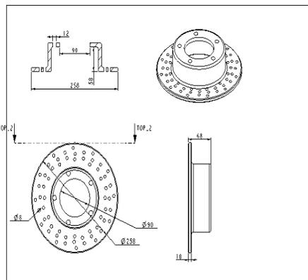
Fig: 10 draft model of a ventilated disc
