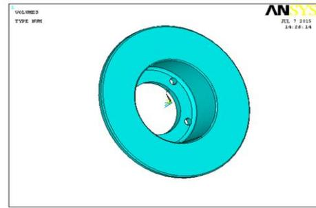
Fig: 11 solid model of a disc brake
