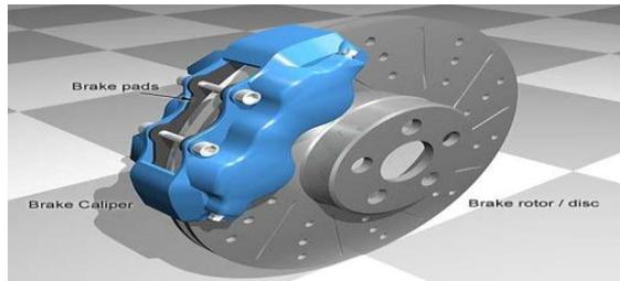
Fig: 1 Disc brake
