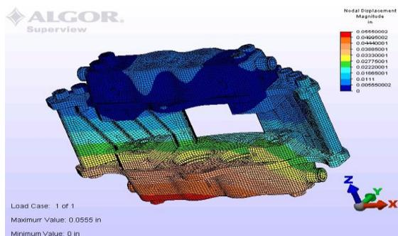
Fig: 7 Overall displacements in the modular caliper
