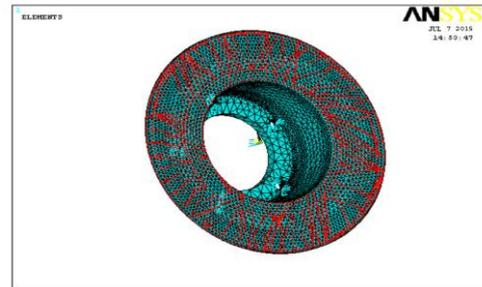
Fig: 12 pressure analysis of a solid disc
