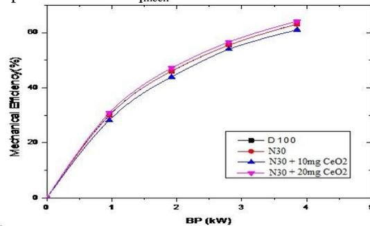
Fig.9. Brake power vs Mechanical efficiency
