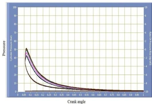
Fig 7. Crank angle vs Pressure at different loads
