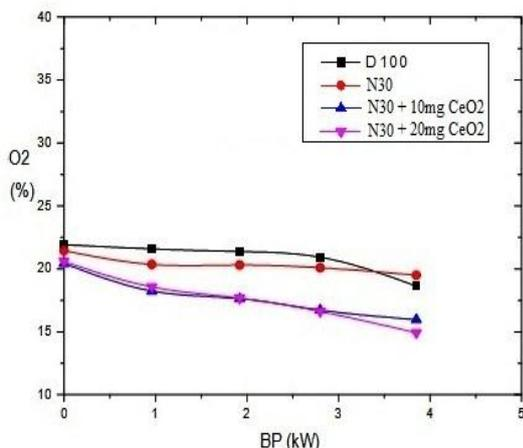
Fig.12. Brake power vs unused oxygen
