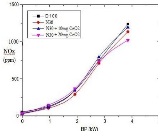
Fig.13. Brake power vs NO<sub>x</sub>
