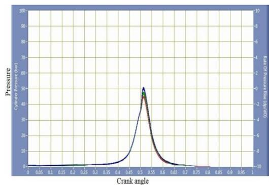
Fig 8. Crank angle vs Pressure at different loads
