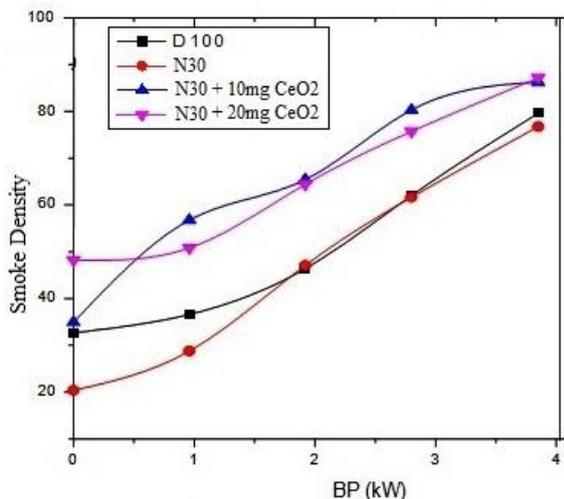
Fig.11. Brake power vs Smoke density
