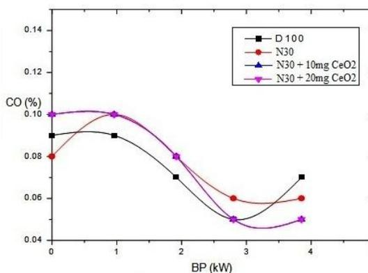
Fig.14. Brake power vs Carbon monoxide
