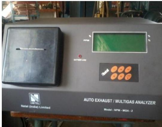
Fig 6: Exhaust gas Analyzer
