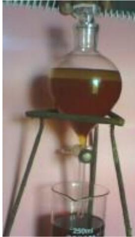
**Fig.3 Process of Separation of Glycerin**
