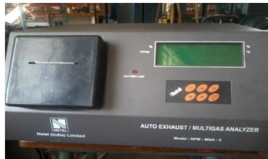
Fig 6: Exhaust gas Analyzer
