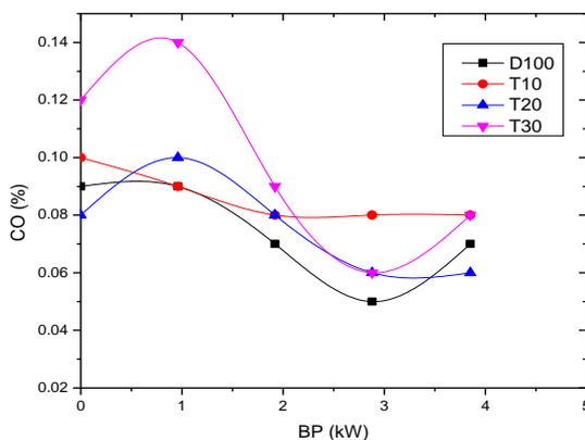
Here the engine exhaust system system is connected to Exhaust Gas Analyser for obtaining the % of CO in exhaust gases at different loads and at different blends. A graph is drawn by taking BP on X-axis and CO on Y-axis. With this graph we can get the information on CO.
