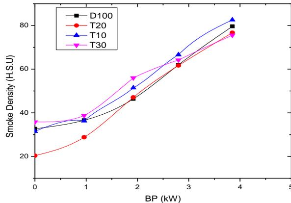
Here the engine exhaust system system is connected to smoke meter for obtaining the smoke density in exhaust gases at different loads and at different blends.A graph is drawn by taking BP on X-axis and Smoke density on Y-axis.With this graph we can get the Max. smoke density .
