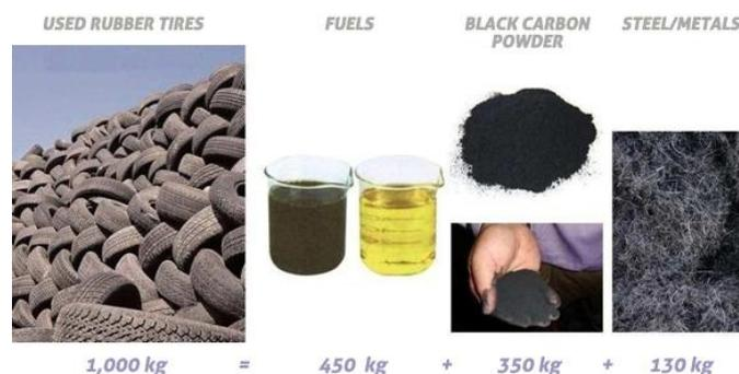
Fig.1: Production of tyre oil.
