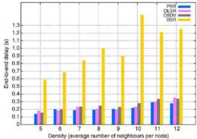
Fig. 4. End-to-end delay in TCP with density.
