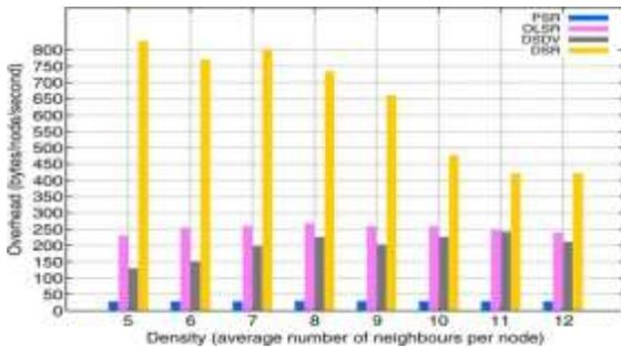
Fig. 2. Routing overhead with density.
