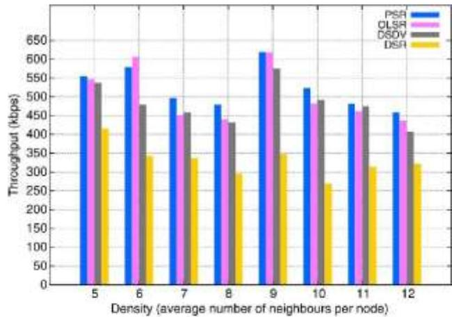
Fig. 3. TCP throughput with density.
