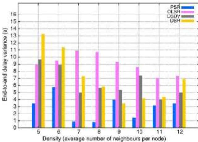
Fig. 9. End-to-end delay in UDP with density.
