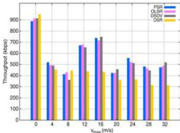
Fig. 5. TCP throughput with velocity
