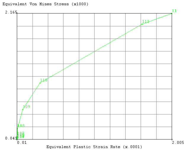
Fig.6 Stress- strain diagram of Ti alloy in conical die at t=5400s
