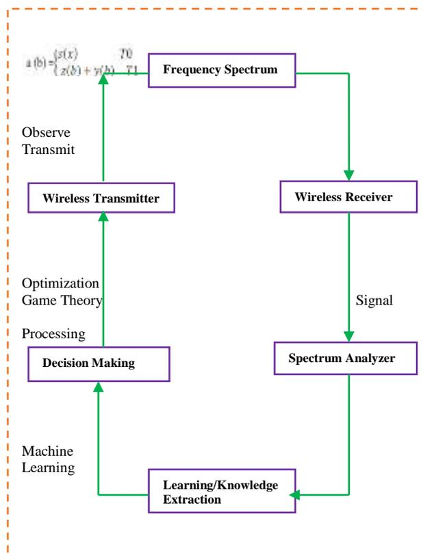
Figure 3: Components of Cognitive Radio Node
