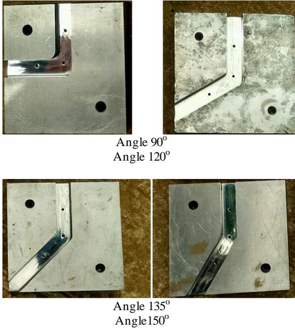
Fig.2 Dies with different angles
