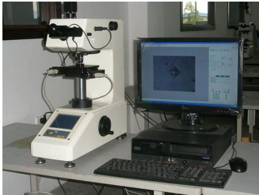
Fig.5 Vickers Hardness Testing Machine
