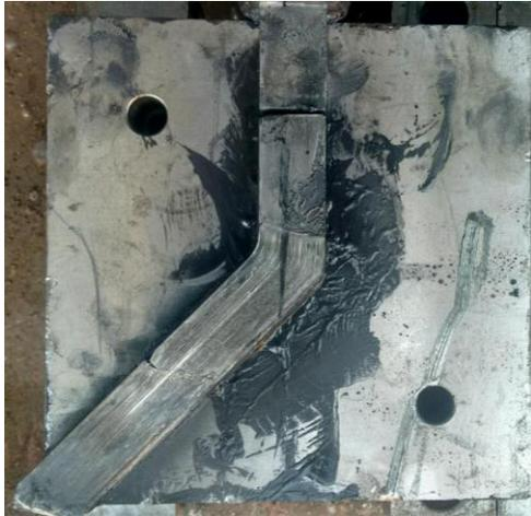
Fig.4 Pressed Specimen
