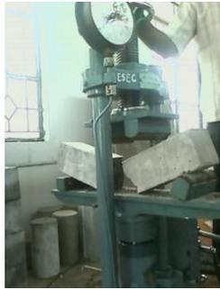
Compression test on concrete Prism
