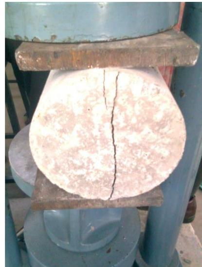
Split Tensile test on concrete Cylinder
