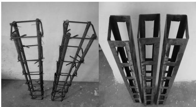
Figure 1. Rebar reinforcement and Prefabricated Cage System
