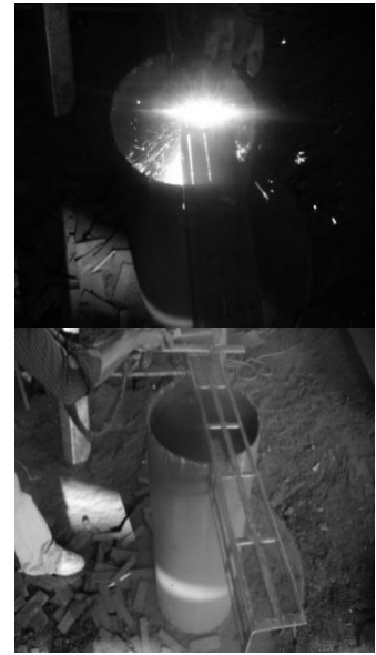
Fig.3. Openings cut by Plasma cutting machine
