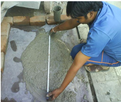
Fig 3 Slump flow test
