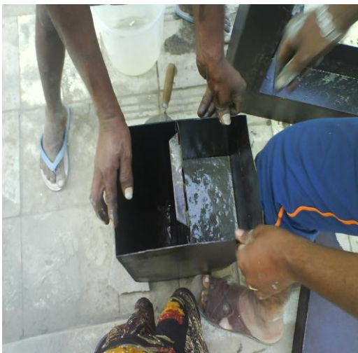
Fig 4 U box test
