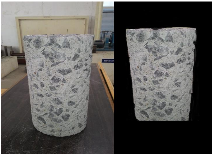
Cylinder and cube after immersed acid curing
