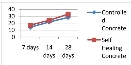
**Figure 1: comparison of compressive strength of Controlled and Auto repairing concrete**
