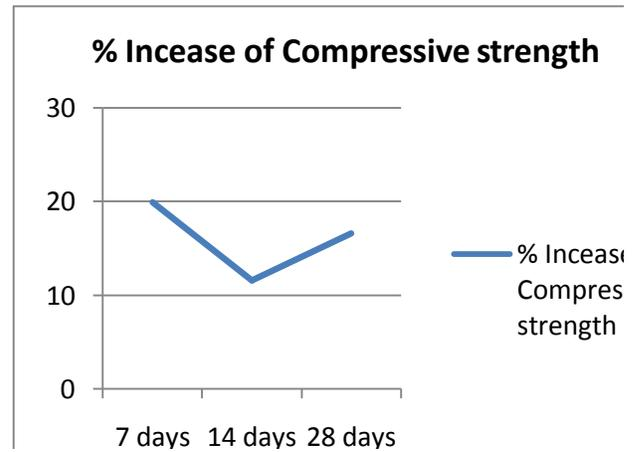
**Figure 3: % Increase in Compressive strength of Auto repairing concrete with ages**
