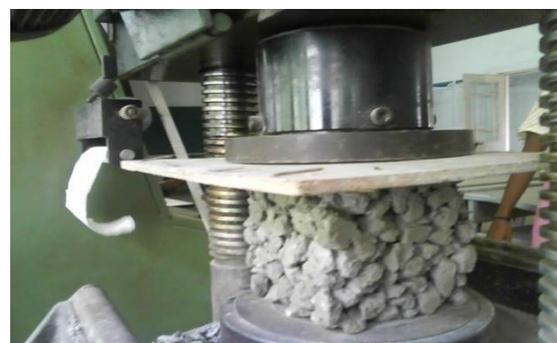
Fig 5.3 Compressive Strength Test
