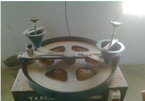
**Fig 5.10 Abrasion testing machine**
