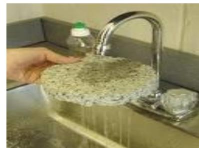
**Fig 5.11 Permeability of pervious concrete**
