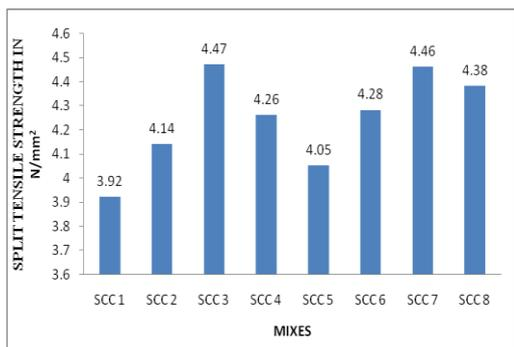
Fig. 8 Split tensile strength at 28 days
