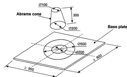
Fig. 1 Slump flow test Apparatus
