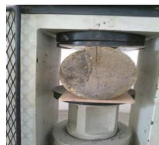
Fig. 7 Split Tensile Test on Cylinder Specimen
