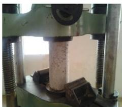
Fig. 9 Cylinder compressive test
