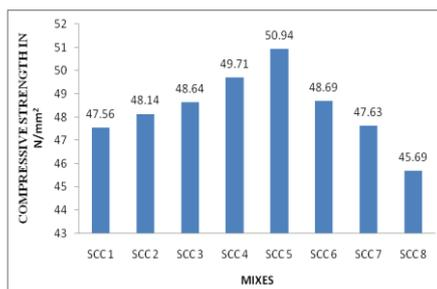
Fig. 6 Cube compressive strength at 28 days
