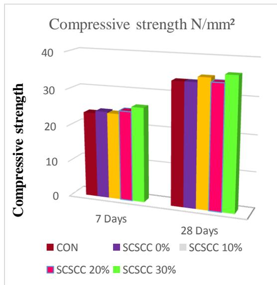
**Fig.3 a) Comparison between conventional and self-compacting self-curing concrete for comp strength test**
