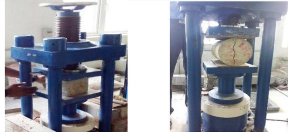
**Fig.2 a) Compressive strength test on cube**
