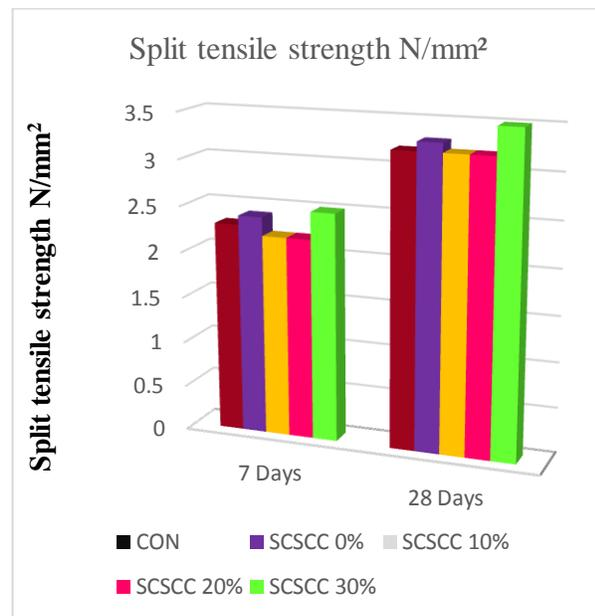
**Fig.3 b) Comparison between conventional and self-compacting self-curing concrete for split tensile strength test**
