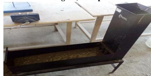
**Fig.1 b) V-Funnel test**
