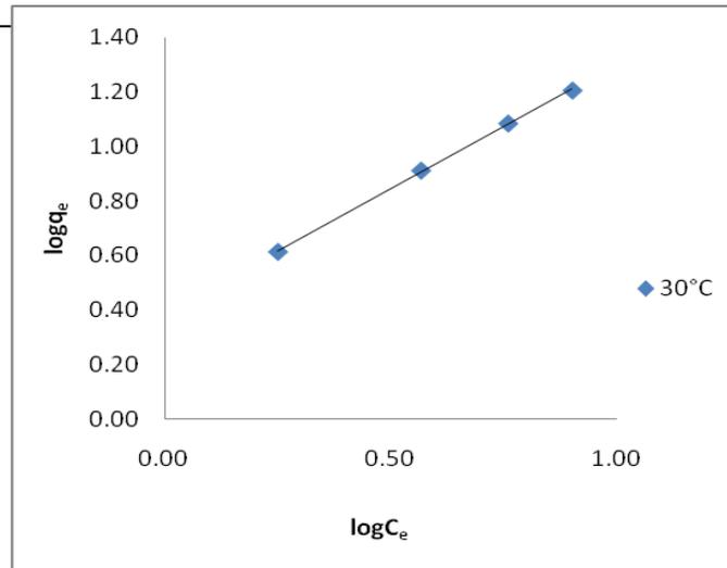
**Fig.2. Freundlich plot for the adsorption of Reactive Red 4 onto AC-MnO<sub>2</sub>-NC**
