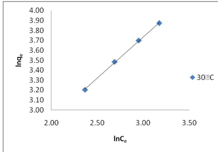
**Fig.5.** Halsey plot for the adsorption of Reactive Red 4 onto AC-MnO<sub>2</sub>-NC
