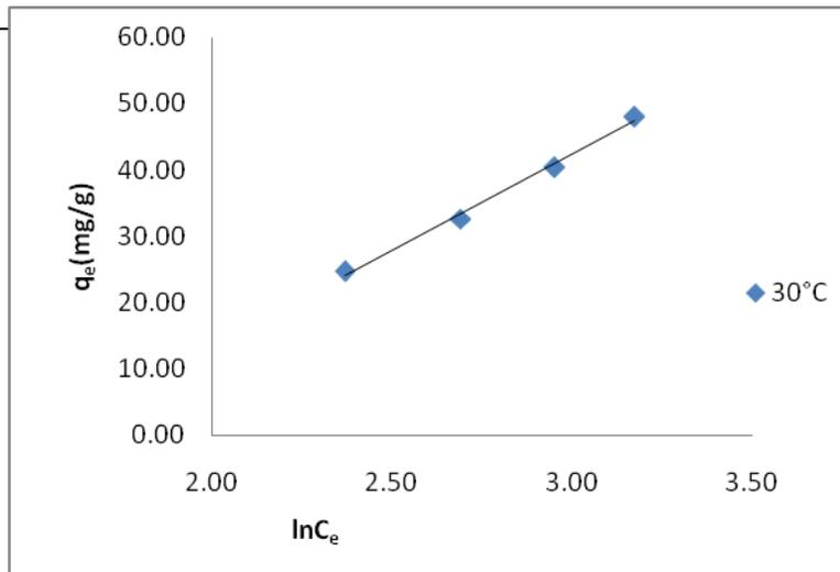
**Fig.3. Temppkin plot for the adsorption of Reactive Red 4 onto AC-MnO<sub>2</sub>-NC**
