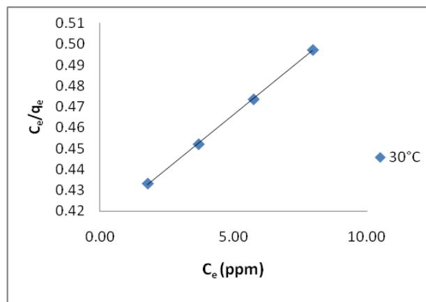
**Fig.1: Langmuir plot for the adsorption of Reactive Red 4 onto AC-MnO<sub>2</sub>-NC**
