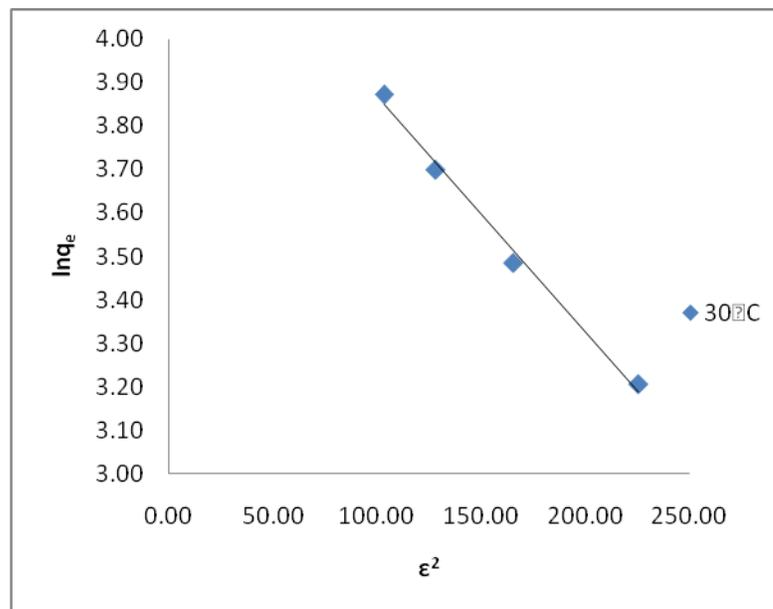
**Fig.4. Dubinin-Radushkevich plot for the adsorption of Reactive Red 4 onto AC-MnO<sub>2</sub>-NC**
