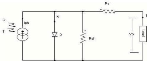
Fig. 1 Equivalent circuit for a solar cell
