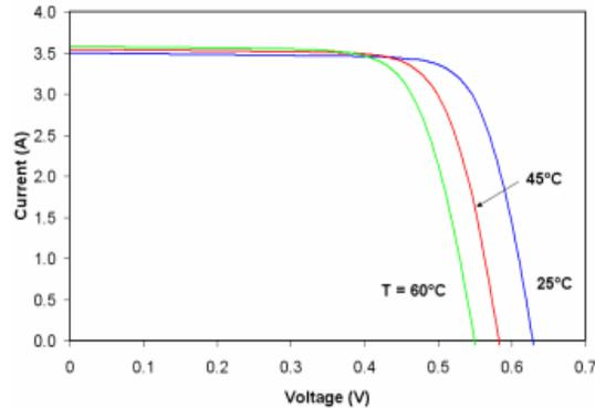
Fig.2 Effect of temperature on the current- voltage
