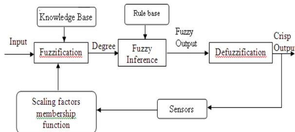
Fig. 4 Functional Block Diagram of FLC
