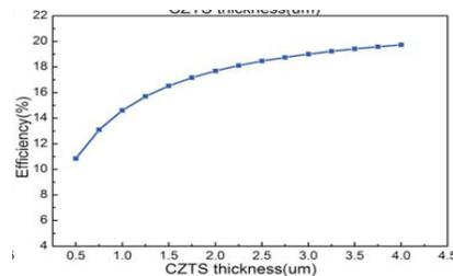
Fig. 4. Efficiency vs thickness of absorber
