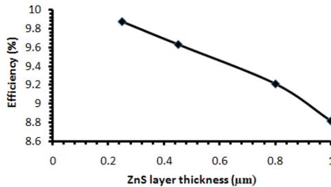
Fig. 7. Efficiency vs thickness of buffer
