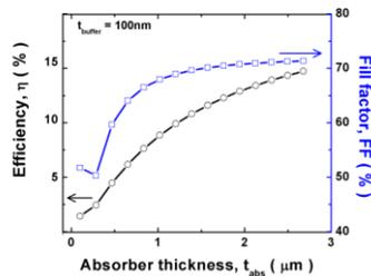
Fig. 8. Efficiency vs thickness of absorber
