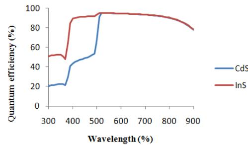
Fig. 3. Spectral response of CdS and In<sub>2</sub>S<sub>3</sub>
