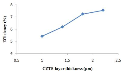
Fig. 1. Efficiency vs thickness of absorber
