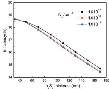
Fig. 5. Efficiency vs thickness of buffer
