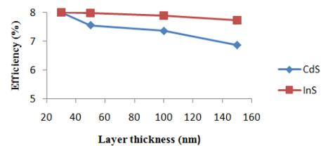
Fig. 2. Efficiency vs thickness of buffer
