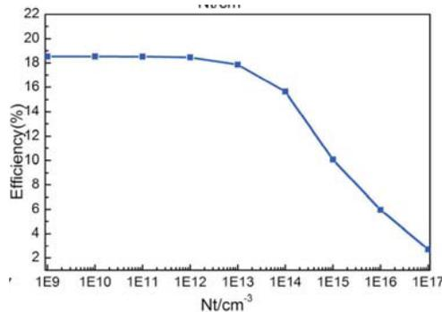
Fig. 6. Cell performance with different defect density
