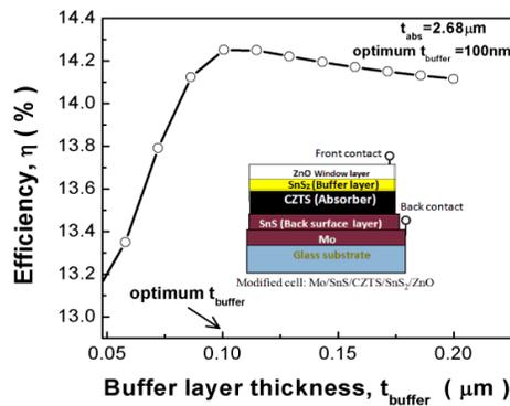
Fig. 9. Efficiency vs thickness of buffer
