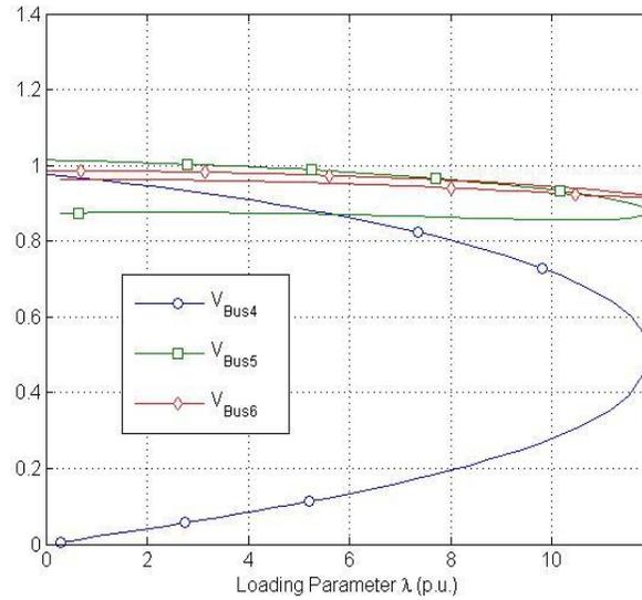
Figure 7. PV curve for 6 bus with TCSC at bus 1 – 45.3.
