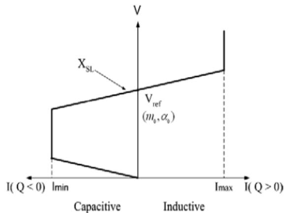
Fig 3b. Characteristic Curve of TCSC
