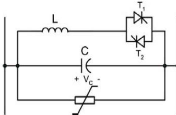
Fig 2. Basic Structure of TCSC
