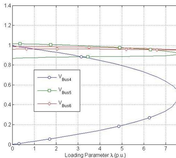
Fig 6. PV Curve of 6 Bus System without FACTS
