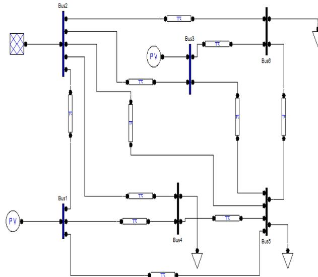
Fig 4. IEEE 6 Bus Test System
