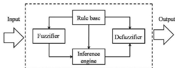
The main idea underlying the fuzzy logic control is, to highlight the issues involved, Fig. 3 shows the basic element of FLC, which comprises four principal components: a fuzzification, a Rule base, Inference engine, and defuzzification.
