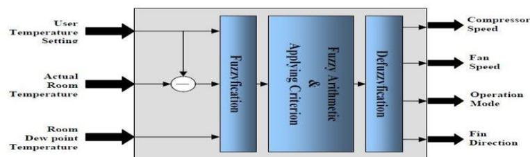
Fig.2. Basic block diagram of controller
