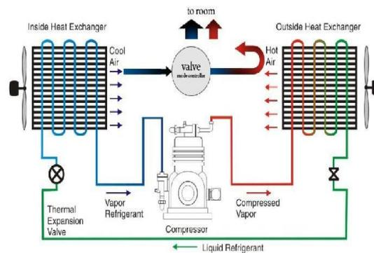
Fig.1. Simplified working diagram of AC
