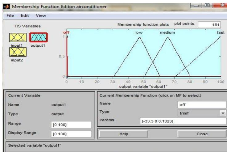
Fig.6. Compressor speed membership functions
