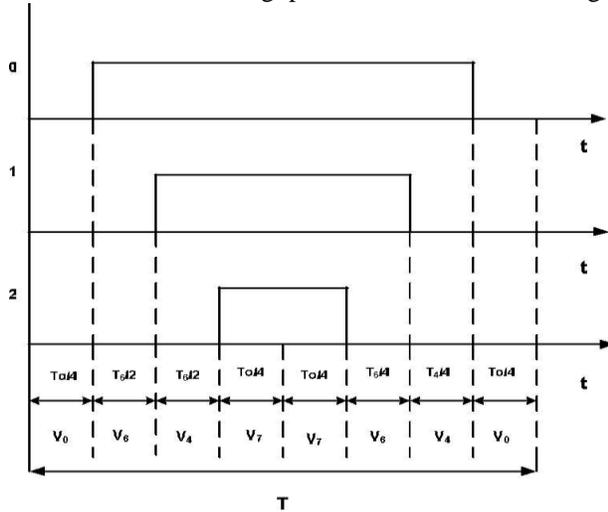
Fig.5 SVPWM switching pattern
