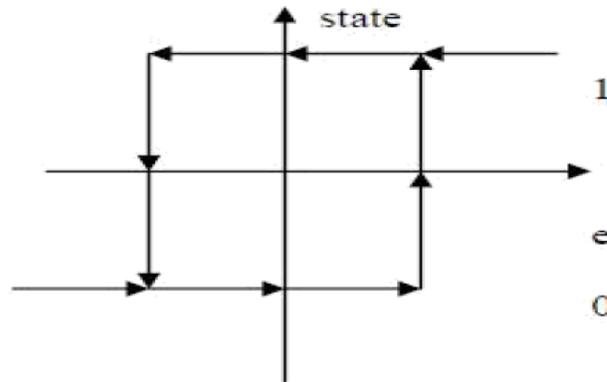
Fig. 3 2-level flux hysteresis comparator
