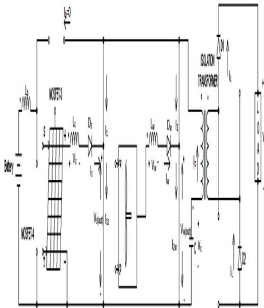
The capacitor will charge when MOSFET1 turned ON in OFF condition capacitor will discharge the power to load through the high frequency transformer, D1 and D2 will conduct. Excess amount of energy is stored in battery through MOSFET3 is in ON condition, at the time battery current  $I_B=0$ .
