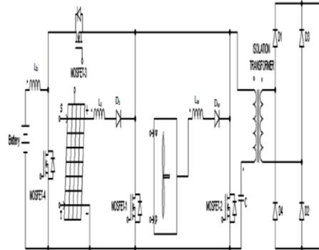
converter has only one switch is connected each input source. In the secondary side of the converter have no controlled switches. The efficiency of the converter is increased by switch ON or switch OFF time interval, depend upon decrease peak current.
